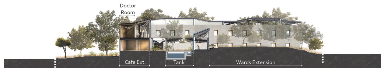
SECTION THROUGH RAINWATER HARVESTING SYSTEM (SECTION C-C')
